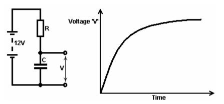
As the voltage increase tails off, it becomes more difficult to measure the difference accurately, so if the capacitor is to be used for generating a time interval, it is normal to use the early part of the graph area where the line is fairly straight and rising fast.
