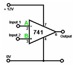
Are you sure you are up to such a difficult circuit? Bit complicated - huh! This is the basic operational form for an operational amplifier.
