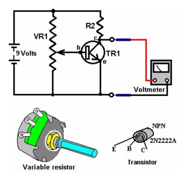
Here we encounter two new components. The first is 'VR1' which is a variable resistor. This device is a resistor which has a slider which can be moved from one end of the resistor to the other. In the circuit above, the variable resistor is connected across the 9 Volt battery so the top of the resistor is at 9 Volts and the bottom is at 0 Volts. The voltage on the slider can be adjusted from 0 Volts to 9 Volts by moving it along the resistor.
