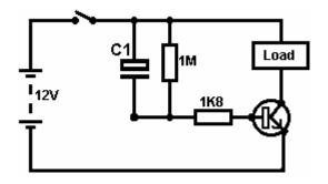
Here, when the switch is closed, both sides of the capacitor C1 are at +12 Volts and this causes the 1K8 resistor to conduct heavily, driving the transistor and powering the load. The capacitor charges rapidly through the transistor and reaches the point at which it can no longer keep the transistor switched on. When the battery is switched off, the 1M resistor discharges the capacitor, ready for the next time the battery is connected.
