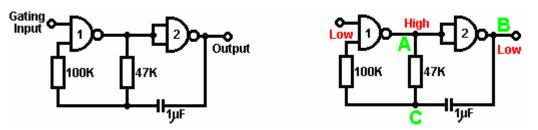
The circuit will not oscillate if the gating input is low, so assume it to be high. Take the moment when the output of gate 2 is low. For this to happen, the inputs of gate 2 have to be high. As the output of gate 1 is wired directly to the inputs of gate 2, it must be high, and for that to be true, at least one of its inputs must be low. This situation is shown on the right.
