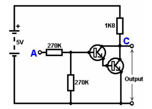
Here, The input impedance has been increased by a factor of 100 by using a Darlington pair of transistors which need far less base current, and so can have a much higher input resistor.
