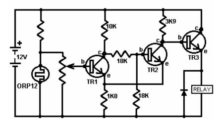
Here, an additional transistor ('TR2') has changed the circuit operation significantly, with transistor TR3 switching fully on and fully off, rapidly. This results in the current through the relay being very low until the circuit triggers.
