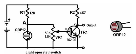
In this version, the voltage at point 'A' controls the circuit. In darkness, the ORP12 has a resistance ten times greater than that of R1 which is 12,000 ohms. Consequently, the voltage at point 'A' will be high. As the light level increases, the resistance of the ORP12 falls, dragging the voltage at point 'A' downwards. As
