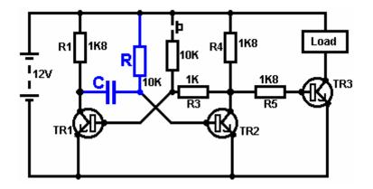
In this circuit, the 'R' resistor and the 'C' capacitor values determine how long the monostable will be in its unstable state. The circuit operates like this:
