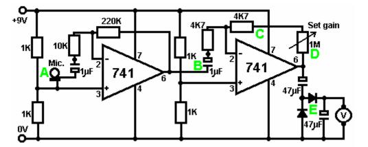
This circuit is two copies of the previous circuit. Each 741 chip has a reference voltage of half the supply voltage created by a voltage-divider pair of 1K resistors. This voltage is fed to pin 3 of the chip, which is the non-inverting input.
