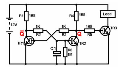
When powered down, the capacitor 'C1' in this circuit is fully discharged through resistor 'R6'. When the 12 Volts supply is connected to the circuit, capacitor C1 does not charge instantly and so holds the base of TR2 down below 0.7 Volts for much longer than it takes for transistor TR1 to switch on (which, in turn, holds TR2 hard off). Mind you, if it is not necessary to have the Load held powered on indefinitely, then an even more simple circuit can do this:
