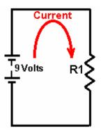
We need to be able to calculate what current is flowing around the circuit. This can be done using "Ohms Law" which states that "Resistance equals Voltage divided by Current" or, if you prefer: "**Ohms = Volts / Amps**" which indicates the units of measurement.
