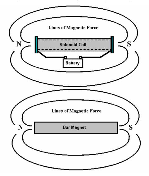
The main difference being that when the current is interrupted, the coil stops acting like a magnet, and that can be very useful indeed. If an iron rod is placed inside the coil and the current switched on, the rod gets pushed to one side. Many doorbells use this mechanism to produce a two-note chime. A 'relay' uses this method to close an electrical switch and many circuits use this to switch heavy loads (a thyristor can also be used for this and it has no moving parts).
