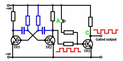
Here, transistors 'TR1' and 'TR2' are connected to form an astable (multivibrator). The astable runs freely, producing the square wave voltage pattern shown in red. Transistor 'TR3' passes this voltage signal on. TR3 inverts the square wave, but this has no practical effect, the output being the same frequency square wave as the signal taken from the collector of TR2.
