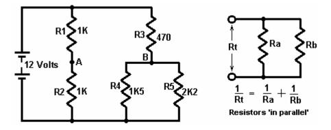
As the current flowing through resistor 'R1' has then to pass through resistor 'R2', they are said to be 'in series' and their resistances are added together when calculating current flows. In the example above, both R1 and R2 are 1K resistors, so together they have a resistance to current flow of 2K (that is, 2,000 ohms).
