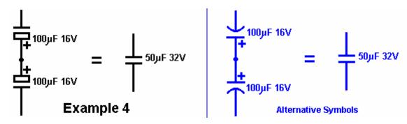
When the capacitors are connected this way, it does not matter which end of the pair is connected to the positive side of the circuit and which to the negative side.
