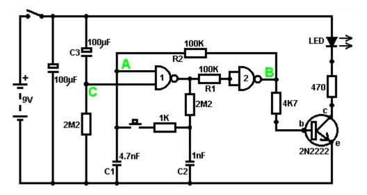
This circuit operates exactly the same way as the previous circuit if, and only if, the voltage at point 'C' is high. With the voltage at point 'C' high, gate 1 is free to react to the voltage at point 'A' as before. If the voltage at point 'C' is low, it locks the output of gate 1 at the high level, forcing the output of gate 2 to the low level and holding the LED off.
