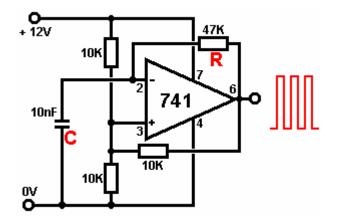
The rate of oscillation of this circuit is governed by the Resistor marked 'R' in the diagram and the capacitor marked 'C'. The larger the resistor, the lower the rate of oscillation, the larger the capacitor, the lower the rate of oscillation.
