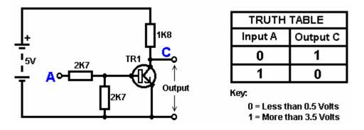
We can see that if the voltage at the input 'A' is taken high, then the output voltage at 'C' will be low. If the voltage at the input 'A' is taken low, then the output voltage at 'C' will be high. A circuit which does this is called an 'Inverter' because it 'inverts' (or 'turns upside down') the input voltage.
