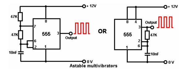
We can also wire the 555 to give a variable mark/space ratio while holding the frequency of the oscillation fixed:
