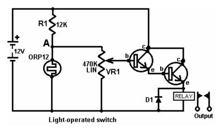
This is almost the same as the light-operated circuit shown earlier. In this variation, the transistors are wired so that they work as an 'emitter-follower' which follows the voltage at point 'A' which rises as the light level drops and the resistance of the ORP12 increases. This causes the voltage across the relay to increase until the relay operates and closes its contacts. A relay is a voltage-operated mechanical switch which will be described in more detail later on.
