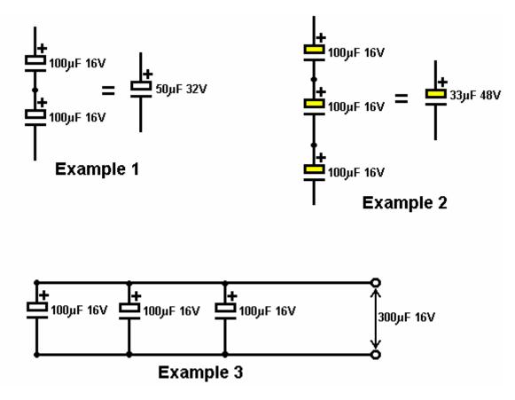
If two capacitors are wired in series, as shown in Example 1 above, the overall capacity is reduced while the voltage rating increases. The reduction in capacitance is given by:
