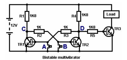
This circuit has two stable states and so it is called a "bi" "stable" or "bistable" circuit. It is important to understand the operation of this simple and useful circuit.
