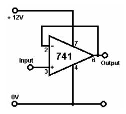
Difficult circuit - huh! Are you sure you can afford all the extra components? This circuit utilises the full gain of the 741 chip. The output follows the input waveform exactly. The input requires almost no current, so the circuit is described as having a 'high input impedance'. The output can drive a serious load such as a relay, so the circuit is described as having a 'low output impedance'.
