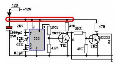
Here, the components just below the diode are ringed to show that they have been marked on the layout sketch and, if necessary, the copper strip broken to isolate the components. A component worth mentioning in passing, is the capacitor marked with red in the circuit diagram. This is a decoupling capacitor, fed from the 12V battery via a resistor and a diode (a diode is not normally used in this part of the circuit).
