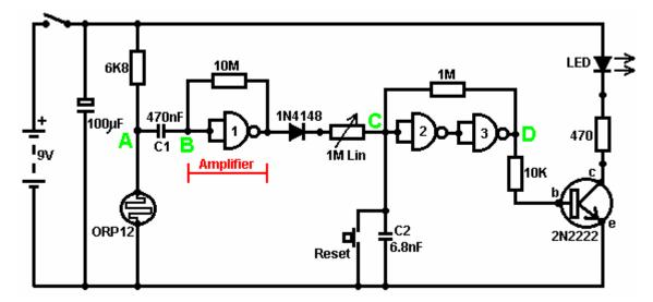
This circuit operates when there is a sudden change in light level. The previous light-level switching circuit was designed to trigger at some particular level of increasing or decreasing level of lighting. This is a shadow-detecting circuit which could be used to detect somebody walking past a light in a corridor or some similar situation.
