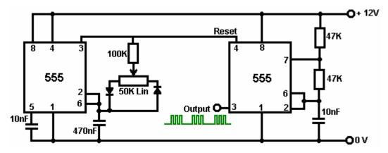
Both of the 555 circuits can be bought in a single 14-pin DIL package which is designated '556'.
