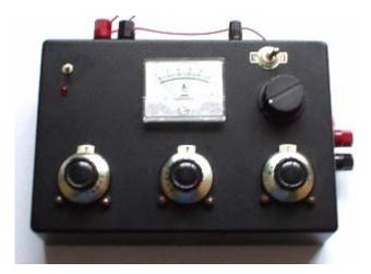
The really essential item of equipment is a multimeter. These come in many shapes, sizes and varieties and the cost varies enormously. The reliability also varies a great deal. The most reliable and the cheapest is the analogue type which does not use a battery (other than for the occasional measurement of resistance). Although these types are looked down upon nowadays, they are 100% reliable:
