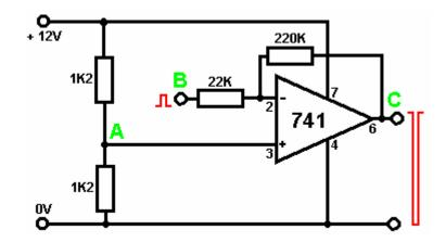
Here, the gain is set by the ratio of the 220K resistor to the 22K resistor. This circuit has a gain of 10 times, so the input signal at point 'B' will generate an output signal at point 'C' which is ten times larger, **provided** that the output signal does not approach the battery voltage. If it does, then clipping will occur with the top and the bottom of the output waveform chopped off at about a volt away from the battery voltage levels, approximately 1 Volt and +11 Volts in this example.
