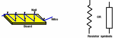
When drawing a circuit diagram, the researcher would sketch the wire on the board giving a zig-zag line which is still used today to represent a 'resistor' although different methods of construction are now used. An alternative symbol for a resistor is a plain rectangle as shown above.
