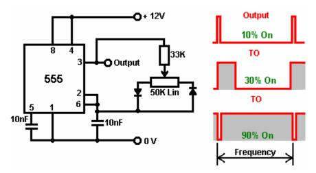
The output waveform changes drastically as the variable resistor is adjusted, but the frequency (or pitch of the note) of the output stays unaltered.
