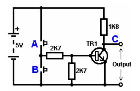
If neither of the press-button switches are operated, the transistor has no base/emitter current flow and so it is off. This places the collector voltage at 'C' near the positive rail (+5 Volts).
