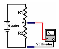
What is the voltage at point 'A'? If you feel like saying "Who cares?" then the answer is "you" if you want to understand how circuits work, because the voltage at point 'A' is vital. For the moment, ignore the effect of the voltmeter used to measure the voltage.
