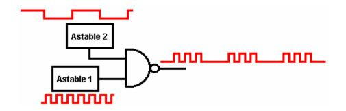
The small circle on the output side of logic devices is to show that they are inverting circuits, in other words, when the input goes up, the output goes down. The two logic devices we have encountered so far have had this circle: the Inverter and the NAND gate.
