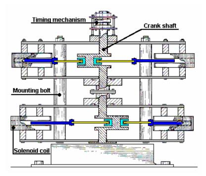
Ben has used eight solenoids to imitate the way that a car engine works. There is a crankshaft and connecting rods, as in any car engine. The connecting rods are connected to a slip-ring on the crankshaft and the solenoids are given a pulse of current at the appropriate moment to pull the crankshaft round. The crankshaft receives four pulls on every revolution. In the arrangement shown here, two solenoids pull at the same moment.
