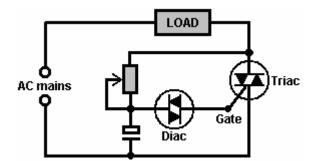
Here, the variable resistor/capacitor pair controls the point on the AC waveform that the Triac is triggered and so controls how much of each sinewave cycle is passed to the mains equipment, and so it controls the average power passed to the equipment. A very common use for a circuit of this type is the 'dimmer-switch' used with household lighting.
