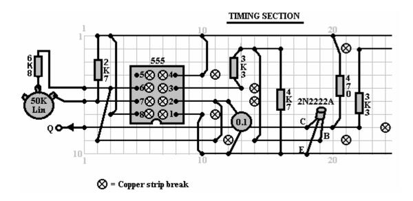
It is very important when producing a sketch like this, that the copper strips making up the circuit are not accidentally used to connect components further along the board, without breaking the copper strip between the two sections of the board. It helps to mark a copy of the circuit diagram when you are sketching a possible physical layout on the stripboard. It might be done like this:
