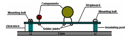
The circuit diagram of the circuit to be built is the starting point. You might wish to draw a light grid of lines to represent the matrix of holes in the stripboard. This helps to visualise the run of the copper strips and the sketch can be made to show the exact number of holes available on the piece of stripboard to be used. The stripboard looks like this:
